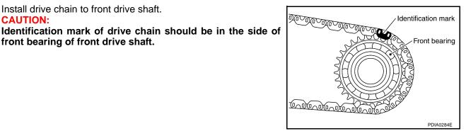
4. Install drive chain to mainshaft, and then install tap front drive shaft with plastic hammer. Press-fit rear bearing of front drive shaft to rear case. **CAUTION:**
