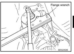
Put matching mark on the end of the mainshaft. The mark should be in line with the mark on the companion flange.
