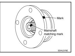
Remove companion flange, using a puller.
