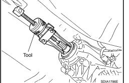
5. Remove the rear oil seal using a puller.
