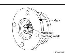
Remove the companion flange using a puller.
