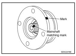
Using flange wrench, install the self-lock nut of companion flange and tighten to the specified torque. Refer to <u>TF-40, "Disassembly and Assembly"</u>.
