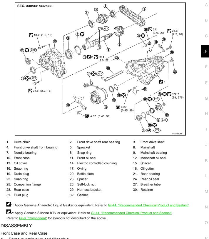
1. Remove drain plug and filler plug.
