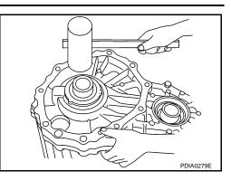
17. Tighten front case and rear case fixing bolts to the specified torque. Refer to "COMPONENTS".
