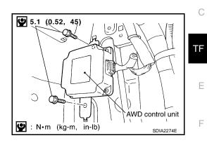
INSTALLATION Install in the reverse order of removal. В
