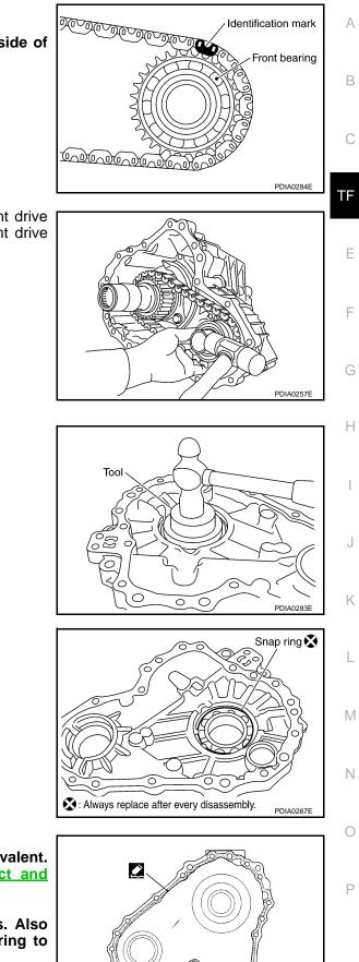
Install drive chain to mainshaft, and then install tap front drive shaft with plastic hammer. Press-fit rear bearing of front drive shaft to rear case.
