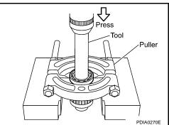
4. Remove front drive shaft rear bearing, using drift and puller.
