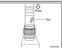
2. Install front drive shaft rear bearing, using a drift.
